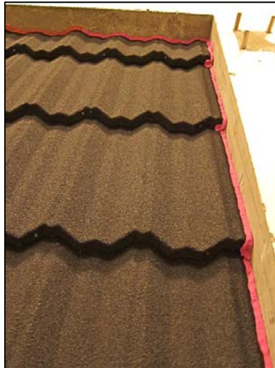
Figure 6: Metal tiles with underlay which were tested with the top row of tiles ending at the top of the concrete opening instead of being bent over.
