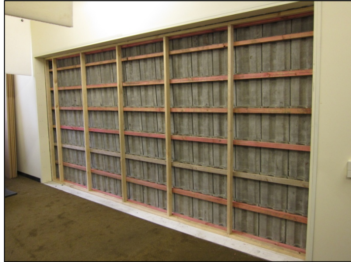
Figure 8: Concrete tiles nailed to battens as viewed from the semi-anechoic room side of the test opening.
