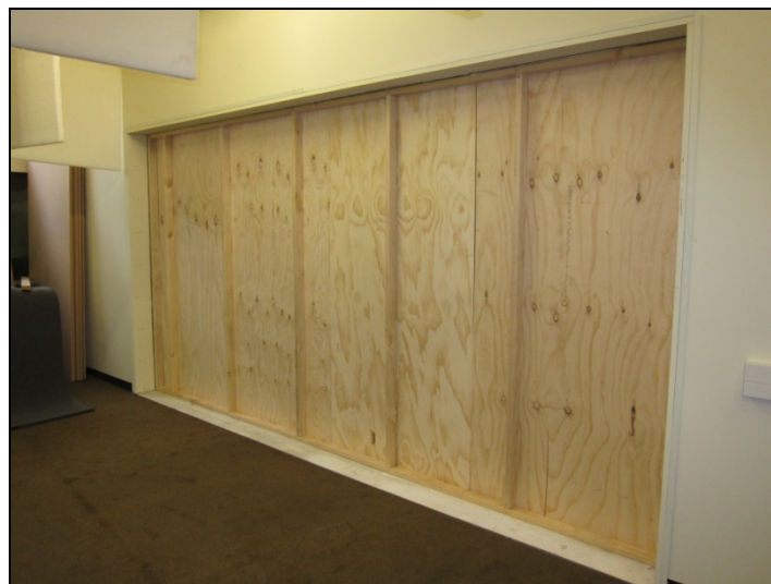
Figure 3: Corrugate 0.4 with plywood sarking as viewed from the semi-anechoic room.
