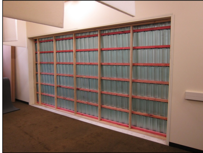
Figure 4: Battens used for the metal tiles as viewed from the semi-anechoic room.
