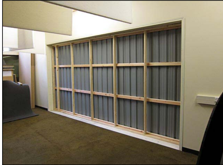
Figure 2: Corrugate 0.4 installed in the test opening as viewed from the semi-anechoic room.
