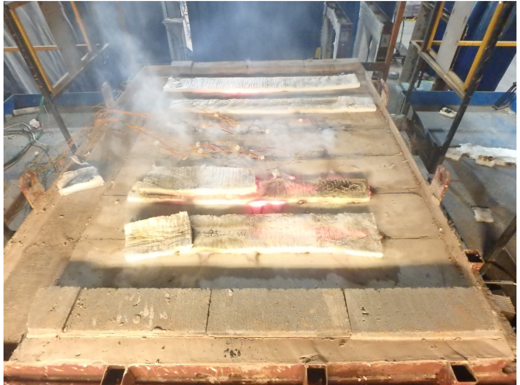
The unexposed face of the floor construction after a test duration of 262 minutes
