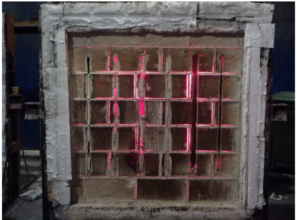
The exposed face of the wall assembly immediately after the test
