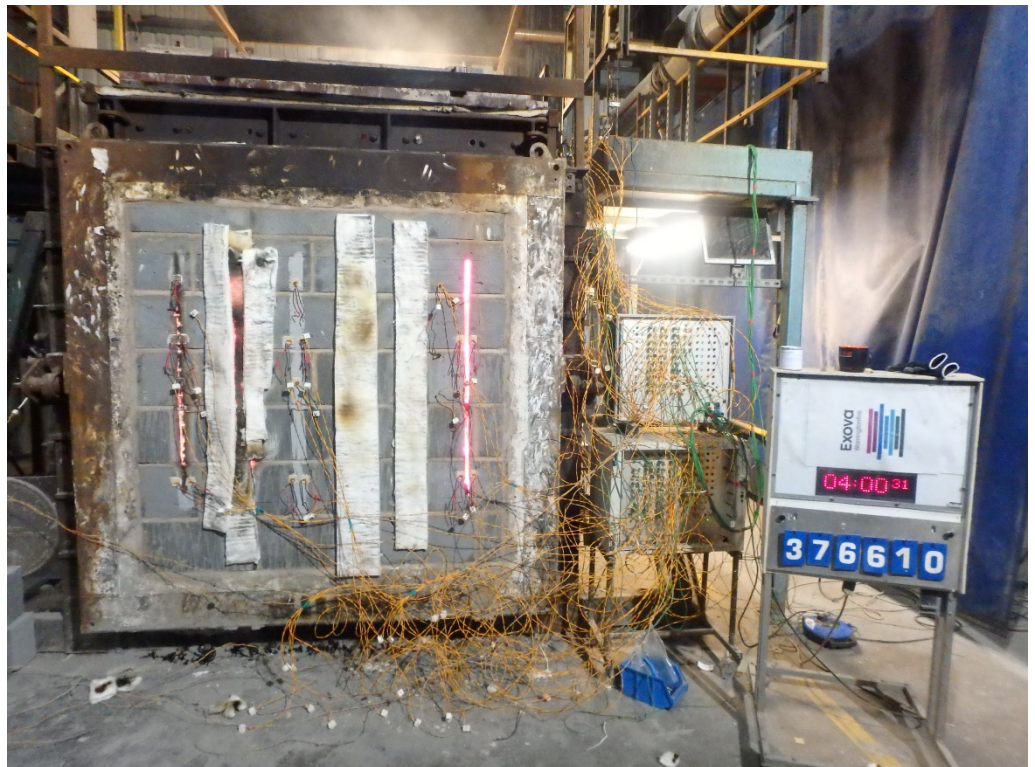
The unexposed face of the wall assembly after a test duration of 240 minutes
