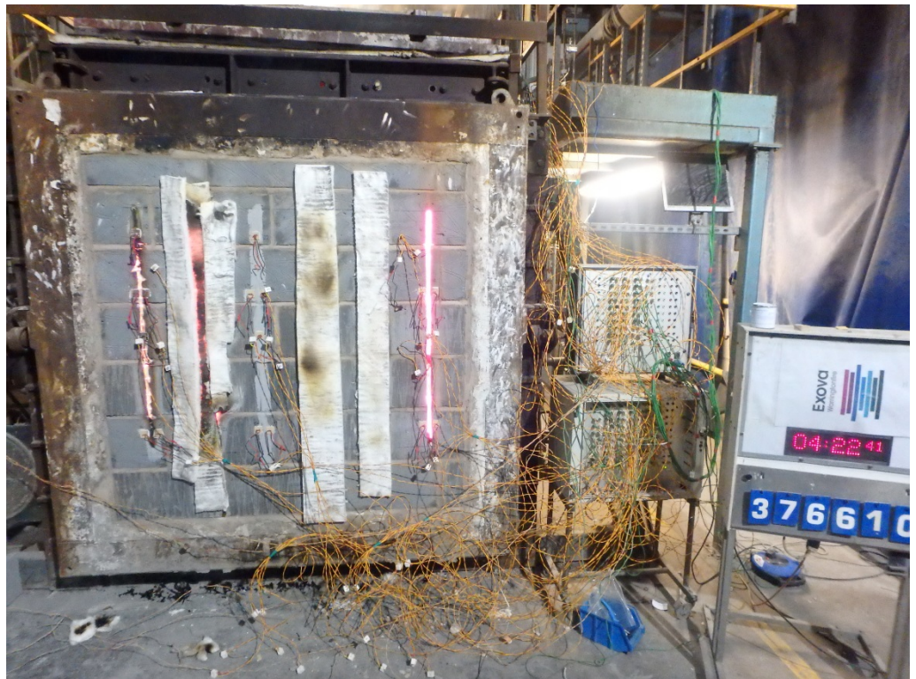
The unexposed face of the wall assembly after a test duration of 262 minutes
