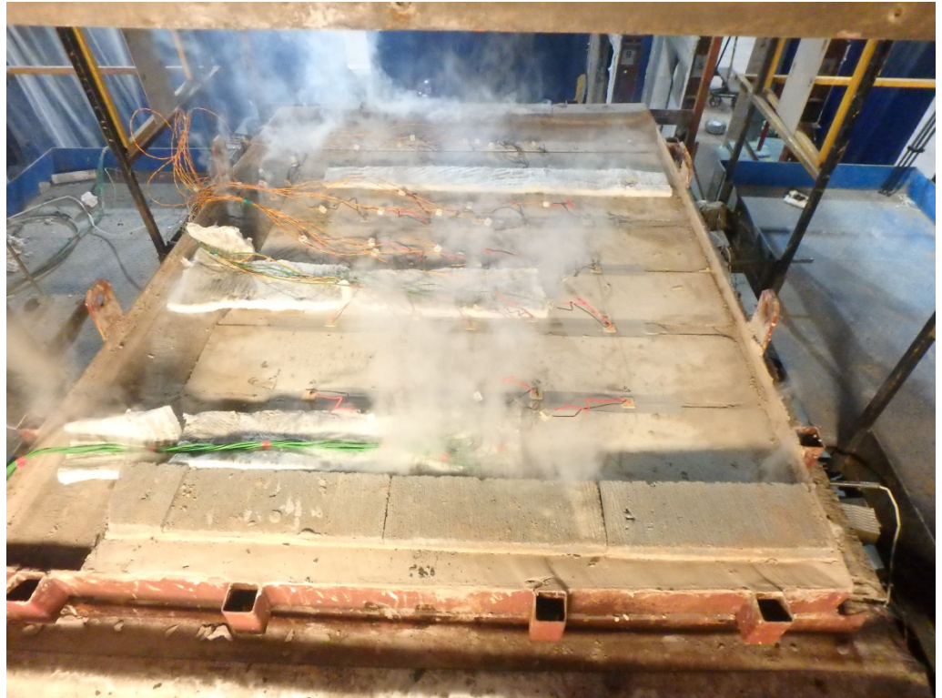
The unexposed face of floor assembly after a test duration of 61 minutes
