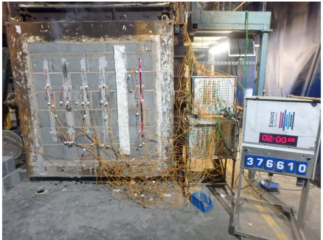
The unexposed face of the wall assembly after a test duration of 120 minutes
