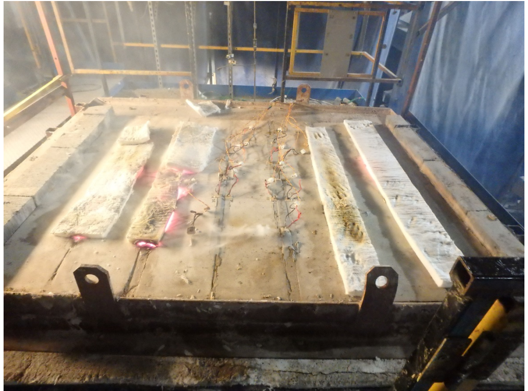
The exposed face of the floor assembly after a test duration of 240 minutes
