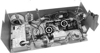
Replace the circuit board (if applicable) and reverse these steps to re-assemble the engine.
