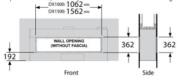
Note: The wall lining directly above the appliance will get warm and hence may discolour paint finishes that are susceptible to temperature damage. The heat may also distort vinyl wall coverings. For durability of finishes and surfaces you should contact the relevant manufacturer for their specification and avoid materials that are not suitable for use above a fireplace.
