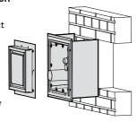
Fit the horizontal powerflue wall terminal into the hole and fix in place, making sure the installation is sealed appropriately to prevent the ingress of water from outside the wall cladding. Take notice of the label on the termination which shows the correct orientation of the terminal.
