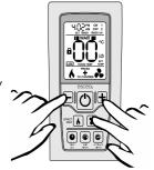
Now hold down the 'EDIT TIMER' and 'ACTIVATE TIMER' buttons simultaneously; the remote display will show the current configuration of either 'NG' for Natural Gas or 'LP' for ULPG/Propane. To change this configuration, hold down the 'EDIT TIMER' and 'ACTIVATE TIMER' buttons simultaneously for 5 seconds. This will now have toggled between gas types.
