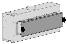
2. Unscrew the firebox rear panel and remove it. Sometimes extra force may be required to remove this panel as the sealing tape can 'glue' itself to the painted surface.
