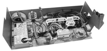
**Step 5:** Remove any screws securing the circuit board to the base and remove the circuit board. Take care that the black spacers underneath the board stay in place until the board is replaced.
