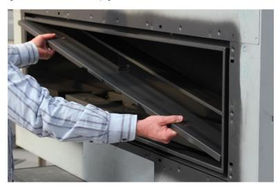
Remove the screws in the bottom and the inner side of the firebox as per shown.
