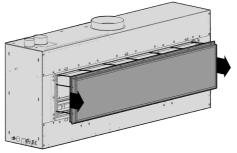
3. Screw the wall lining trim brackets on to the appliance chassis as shown in photo.
