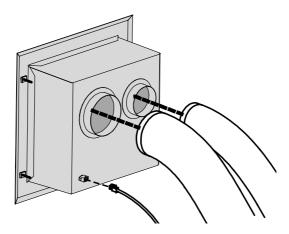
Fit the horizontal powerflue wall terminal into the hole and fix it in place, making sure the installation is sealed appropriately to prevent the ingress of water from outside the wall cladding.
