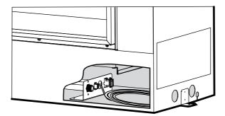
If you do not wish to connect the fireplace to the modem, the Network / Ethernet cable should be run to somewhere accessible by a service technician, such as a cupboard. G
