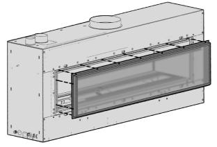
Pull the top of the frame toward you slightly and lift the glass and frame out and away from the fire. Place the glass & frame carefully aside.
