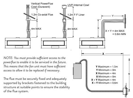
Any joints within the flue system must be sealed adequately with a sealing agent used if necessary. The flue system for the DX1500 / DX1000 is zero rated, so no spaces are required between the flue and any timber framing.
