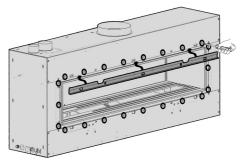
4. Carefully install the extra glass panel and frame onto the appliance, ensuring that the glass does not fall from the frame. Tighten the bolts around the outside of the glass retainer until securely fitted.
