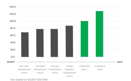
Villaboard Lining's resistance to hard body impact is much greater than other commonly used materials. It was also observed that the area of damage was larger on the impact of other substrates than was observed on Villaboard Lining (where it was confined to an easily repairable crack or small indentation). Again, this is due to Villaboard Lining's uniformly strong composition.
