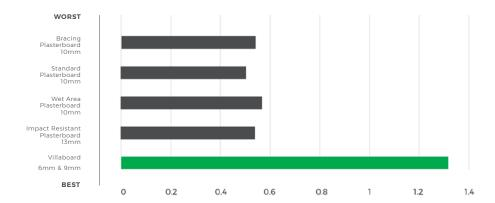
The Standard AS2358 - 'Adhesives - For fixing ceramic tiles', states that a tile adhesive must produce greater than or equal to 0.5MPa (ultimate stress). Compared to the other commonly available materials, Villaboard Lining has greater tile adhesion and hold capacity in dry conditions.
