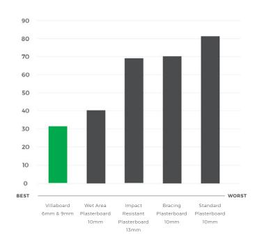
Tested at the James Hardie Research and Development Centre based on 48 hour water absorption of the substrate lining.
