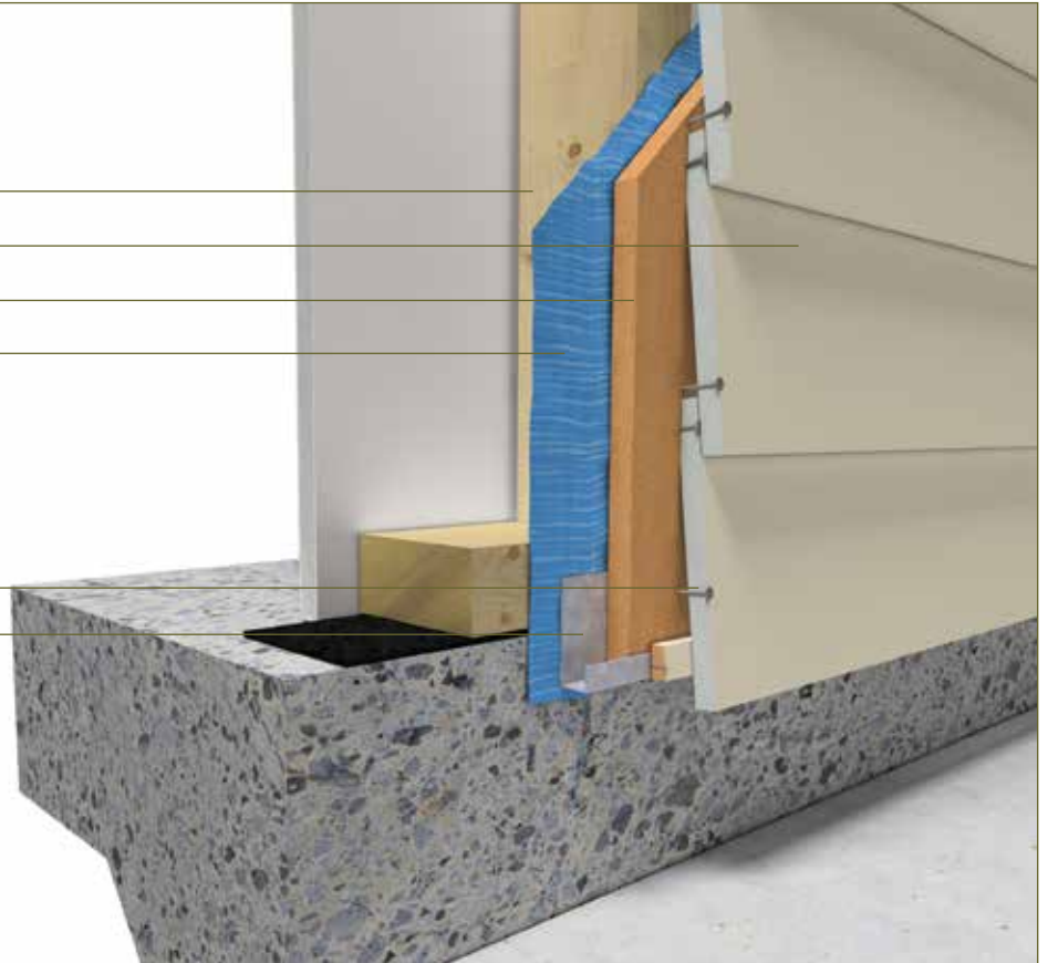
FIGURE 6 FASTENER DETAIL TIMBER FRAMING FACE FIXING SYSTEM
