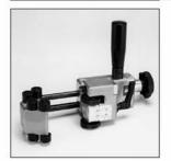
For the safe removal of the oxidic layer on HD-PE and PE-X pipes. Scraper tool made from hard metal (long service life). Includes one replacement blade.
