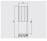
Connection unit between the ready made concrete inspection chamber and the FRIAFIT® sewage insert sleeve (AEM). With anchoring ribs across the whole width of the diameter for a secure seat in the concrete. Resilient centre section serves to take up the stresses when the pipes are under load. Stable inside diameter due to high wall thickness giving a good connection to the AEM in accordance with DIN 4034.
