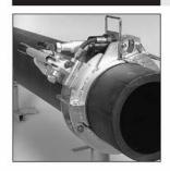
For rerounding of HD-PE and PE-X pipes. We also provide these hydraulic rounding clamps for hire. Prices on request.
