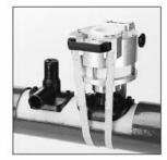
For compressing and providing the required joint pressure. For flexibly matching all FRIALEN® Saddle Components of the TL type to all pipe diameters in the stated range.
