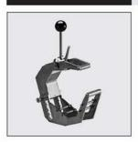
For safe removal of oxidic layer in saddle area on HD-PE and PE-X pipes. Scraping all around not necessary. Extra wide scraper tool made from hard metal. Dimension setting with fast catch. Moveable blade mount to compensate for unevenness of pipe. Includes replacement scraper blade and oil based care spray.
