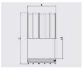
Jointing element between masoned canal and FRIAFIT® AEM sewage insert sleeve. Fixing supports across the entire width for proper fit in canal with retrospective installation. Elastomere central piece to counterbalance stresses. Solid internal diameter due to large wall thickness.
