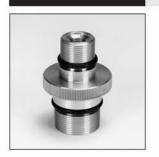
For connection of pressure gauge to carry out pressure check on FRIALEN® pressure tapping valves DAA, DAP, DAA-TL, DAA-TL/RE d1=61-315 (see FRIALEN® price list). Connection dimension female thread = R 1/4".
