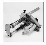
For the safe removal of the oxidic layer on spigot fittings. In addition, it is possible to scrape HD-PE and PE-X pipes (up to a maximum half of coupler length). Scraper tool made from hard metal (long service life). Includes one replacement blade and oil based care spray.
