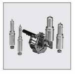
For safe removal of oxidic layer on HD-PE and PE-X pipes and on DAA, DAV, SA, TA T-pieces outlets etc. (see also FRIALEN price list). Guidance/rotation on adjustable extension pins (d32, d40, d50, d63). Scraper tool made from hard metal. Dimension adjustment with fast catch. Sprung blade mount to compensate for pipe ovality. Includes replacement blade and oil based care spray.
