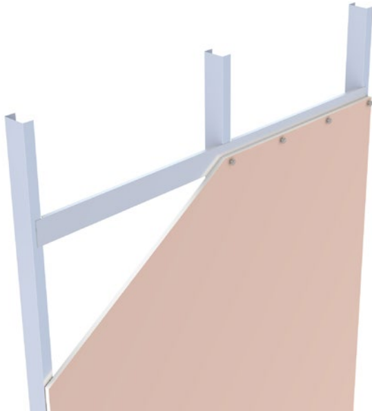
Nog on edge from ex 64mm x 30mm BMT track. Stagger nogs by at least 400mm on opposite sides of the wall.
