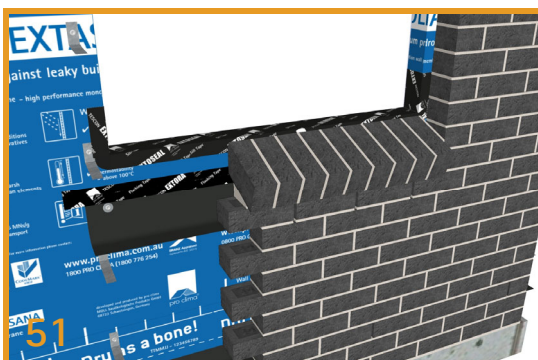
Set the Flashing as per Sill Details Be sure to set the flashing at the correct height to drain to the sill weep holes. TESCON EXTORA® cannot be removed once adhered.
