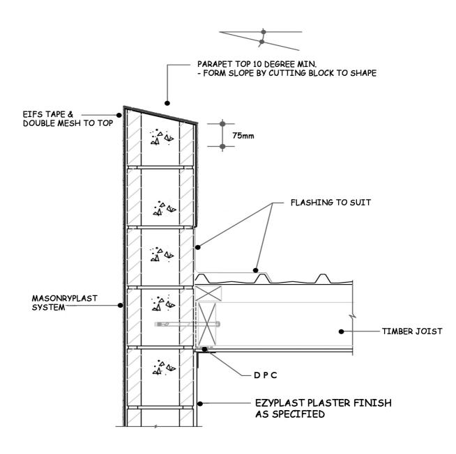
PARAPET WALL / ROOF / DECK DETAIL
