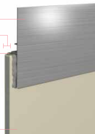
FIGURE 4 BACKING STRIP INSTALLATION - REAR VIEW
